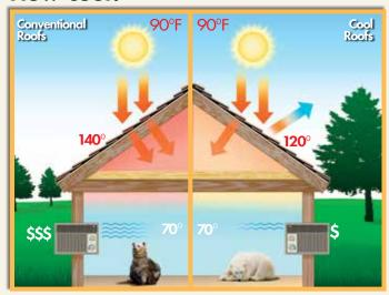
Thanks to the reflective nature of Timberline® Cool Series® Shingles, part of the heat radiating from the sun gets reflected, helping to reduce the heat in the attic and heat going into the house. It may translate into savings on air-conditioning bills.<sup>3</sup>
